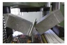
testing machine. Flexural quality is discovered utilizing focus point stacking framework. The example is situated in the gear so that the weight is put on the best surface as cast inside the shape. The
